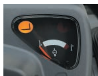
Lifting interlock lamp on the control panel
